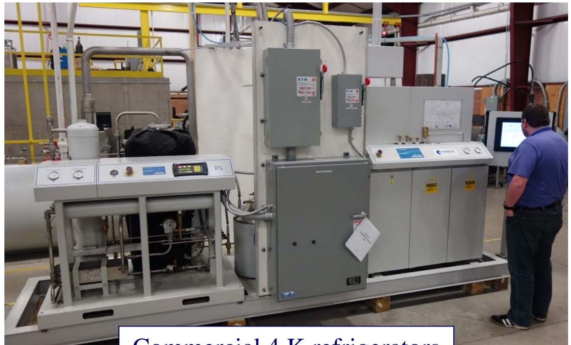
Commercial 4 K refrigerators (rugged piston-based systems, 110 W cryogenic capacity)
